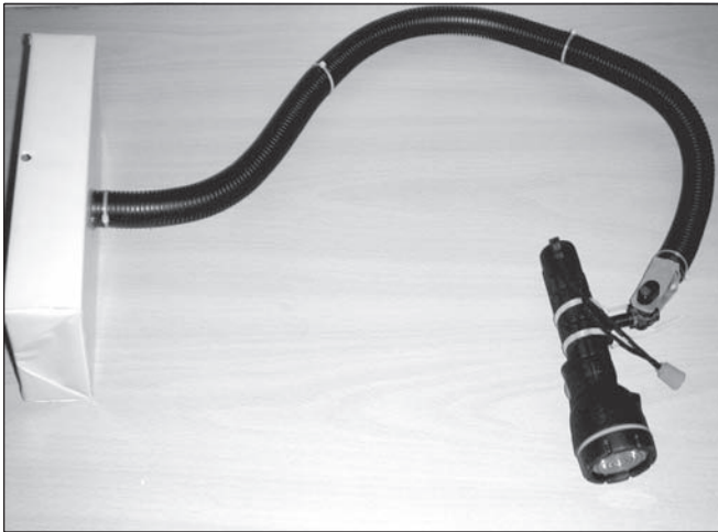
Figure 2. The flashlight was fastened to a gooseneck attached to a gauge -15 galvanized-iron base.
