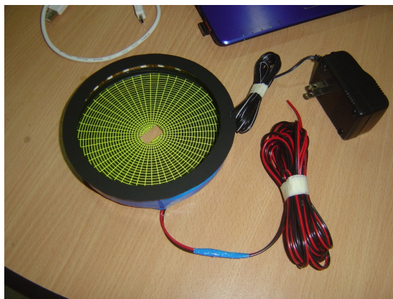
Figure 2. Assembled prototype xeroscope powered by a multi-voltage AC-DC power adapter set at 6-volts and 350mA (2 watts).
